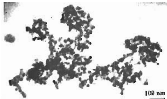
Figure 6.2: TEM micrograph of silver nanoparticles synthesized by inert gas condensation method, used in this study
